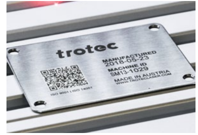
Annealing on stainless steel
